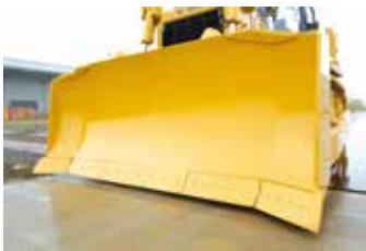
Semi-Universal blade (with hydraulic tilt)
